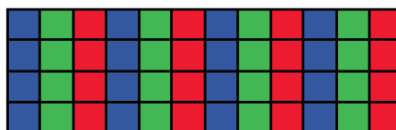
Band-interleaved-by-pixel (BIP) with three bands 12 columns by 4 rows
